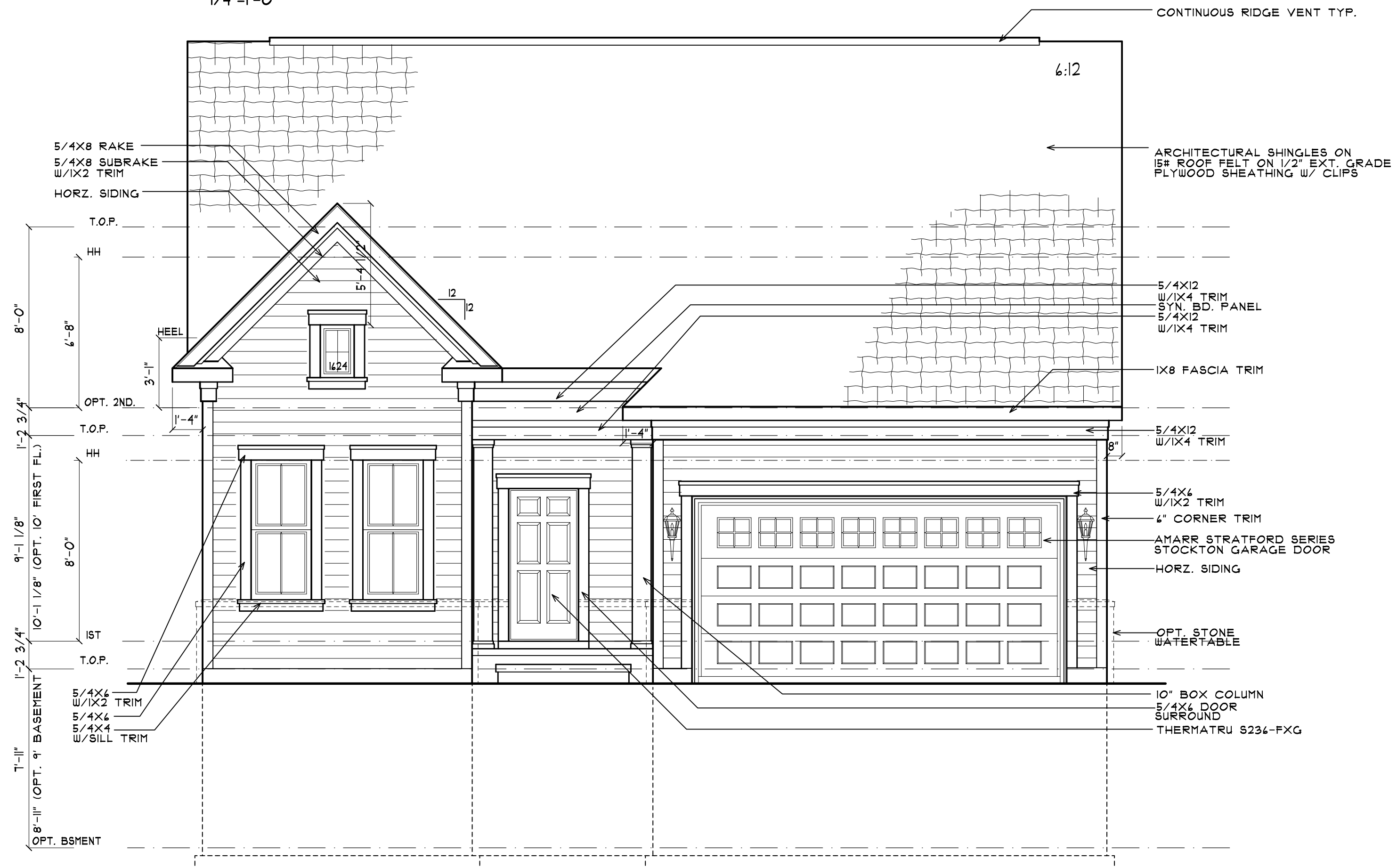
FRONT ELEVATION #1 w/OPT. BASEMENT
