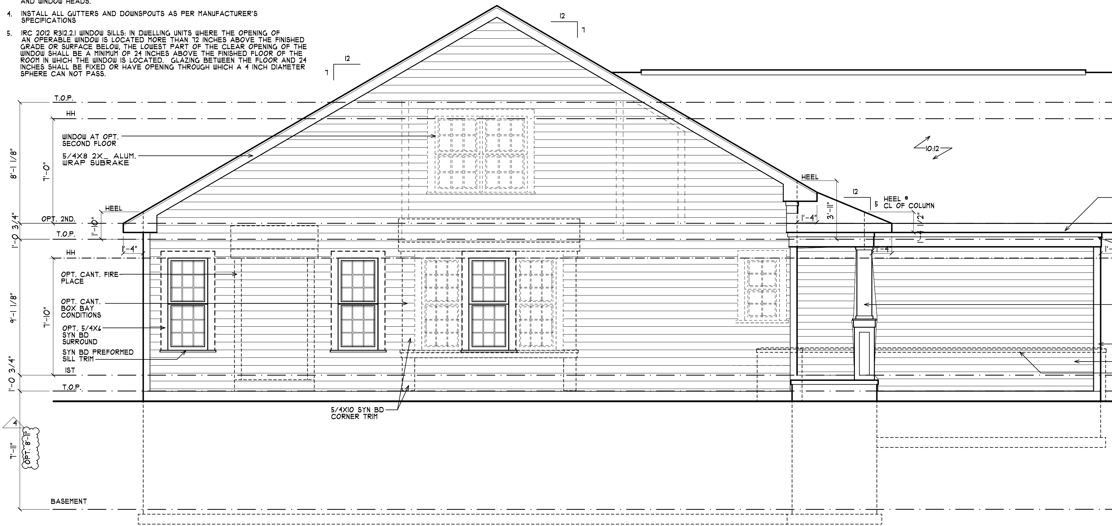
LEFT ELEVATION #1 W/OPT. BASEMENT 1/4"=1'-0"
