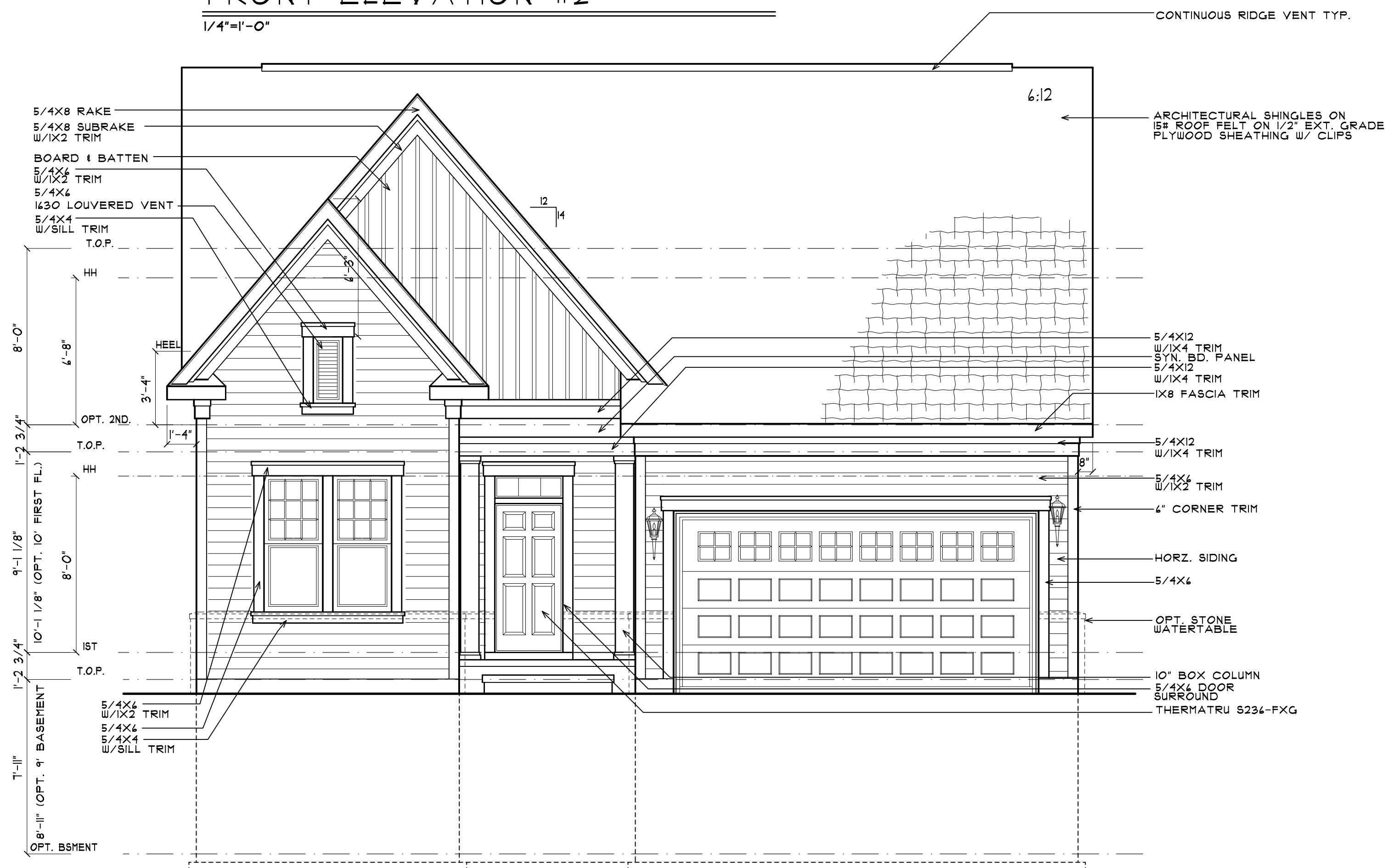
FRONT ELEVATION #2 W/OPT. BASEMENT
