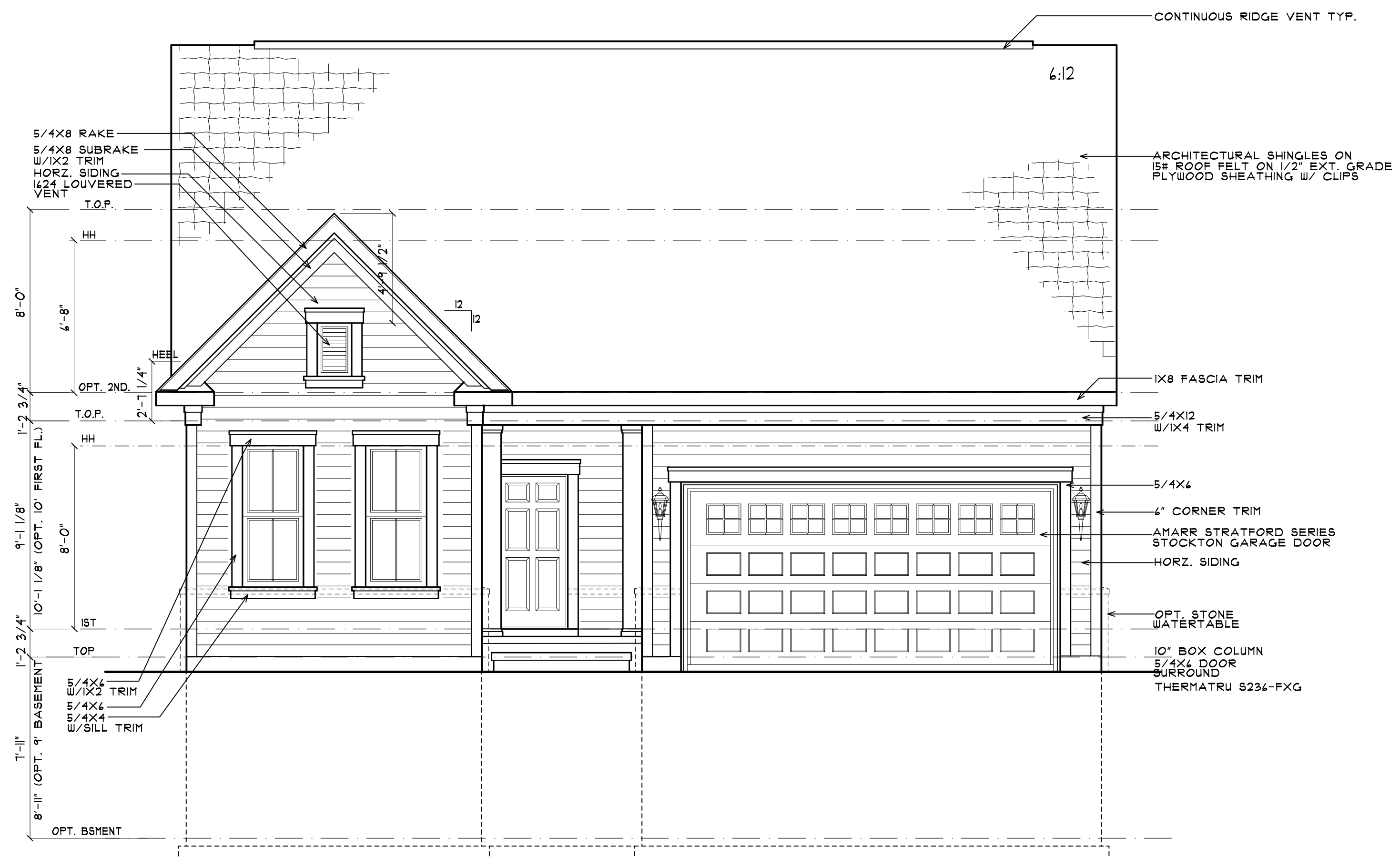
FRONT ELEVATION #1 W/OPT. BASEMENT
