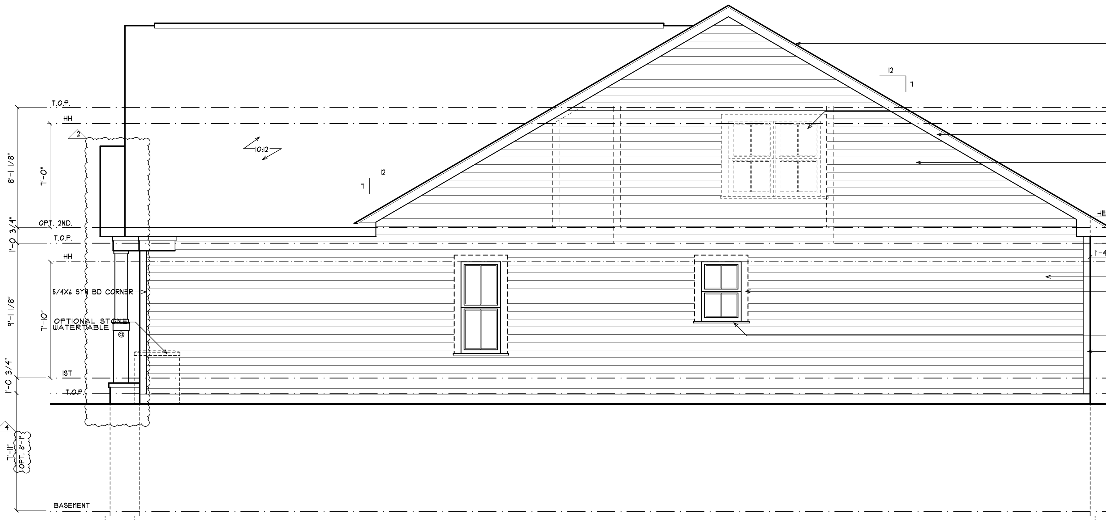
RIGHT ELEVATION #3 W/OPT. BASEMENT 1/4"=1'-0"
