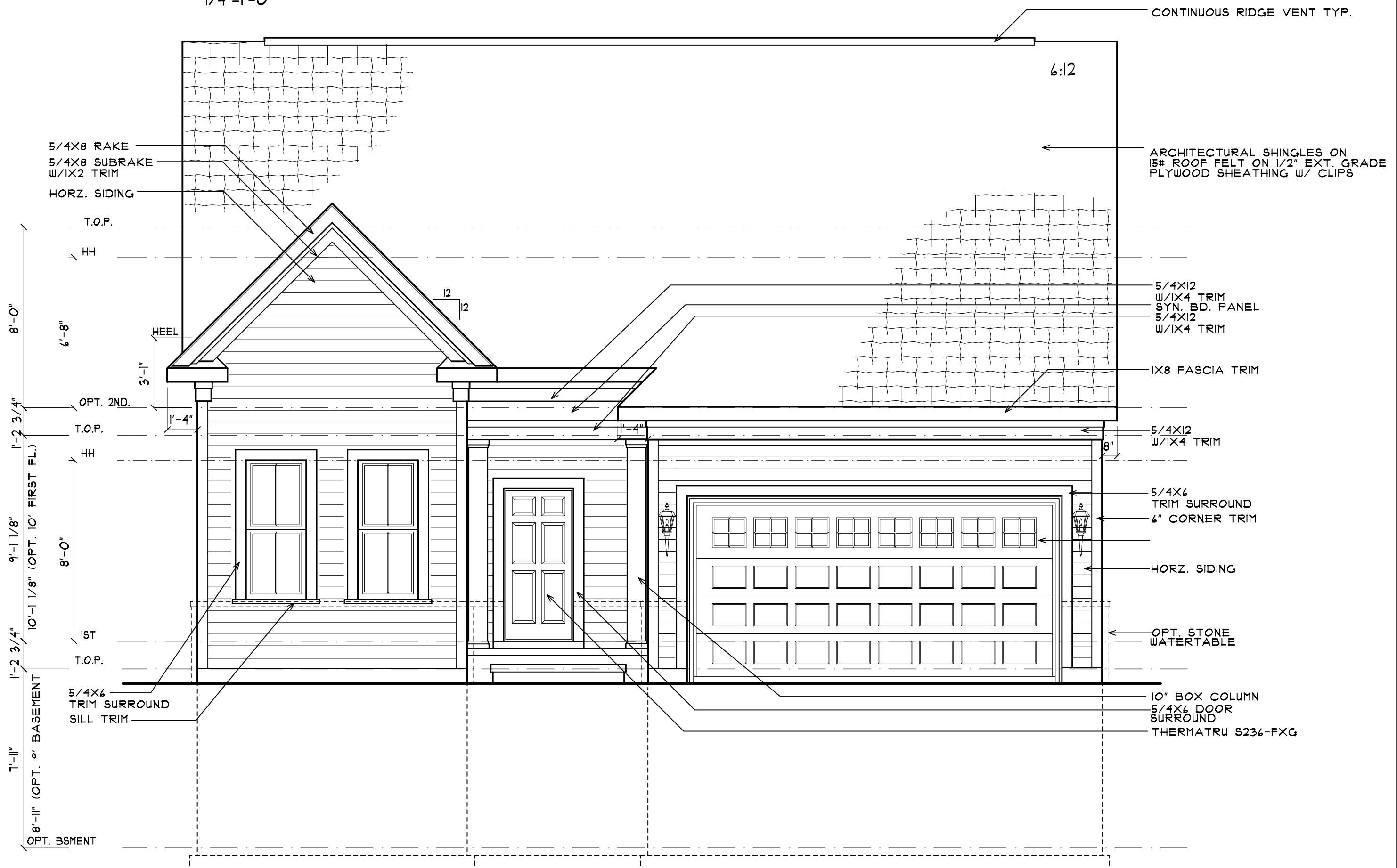
FRONT ELEVATION #0 w/OPT. BASEMENT
