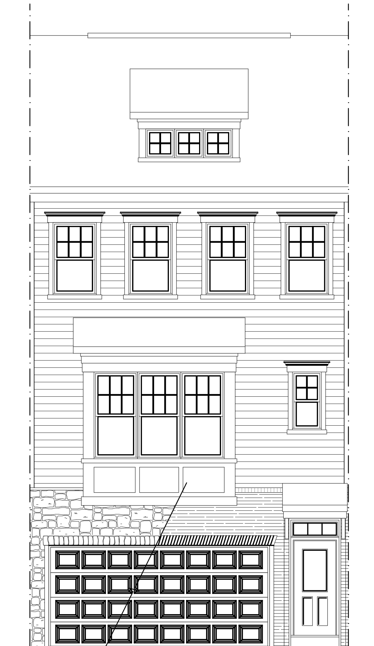
ELEVATION #5 UNIT 2450 1/3 BRICK/STONE
