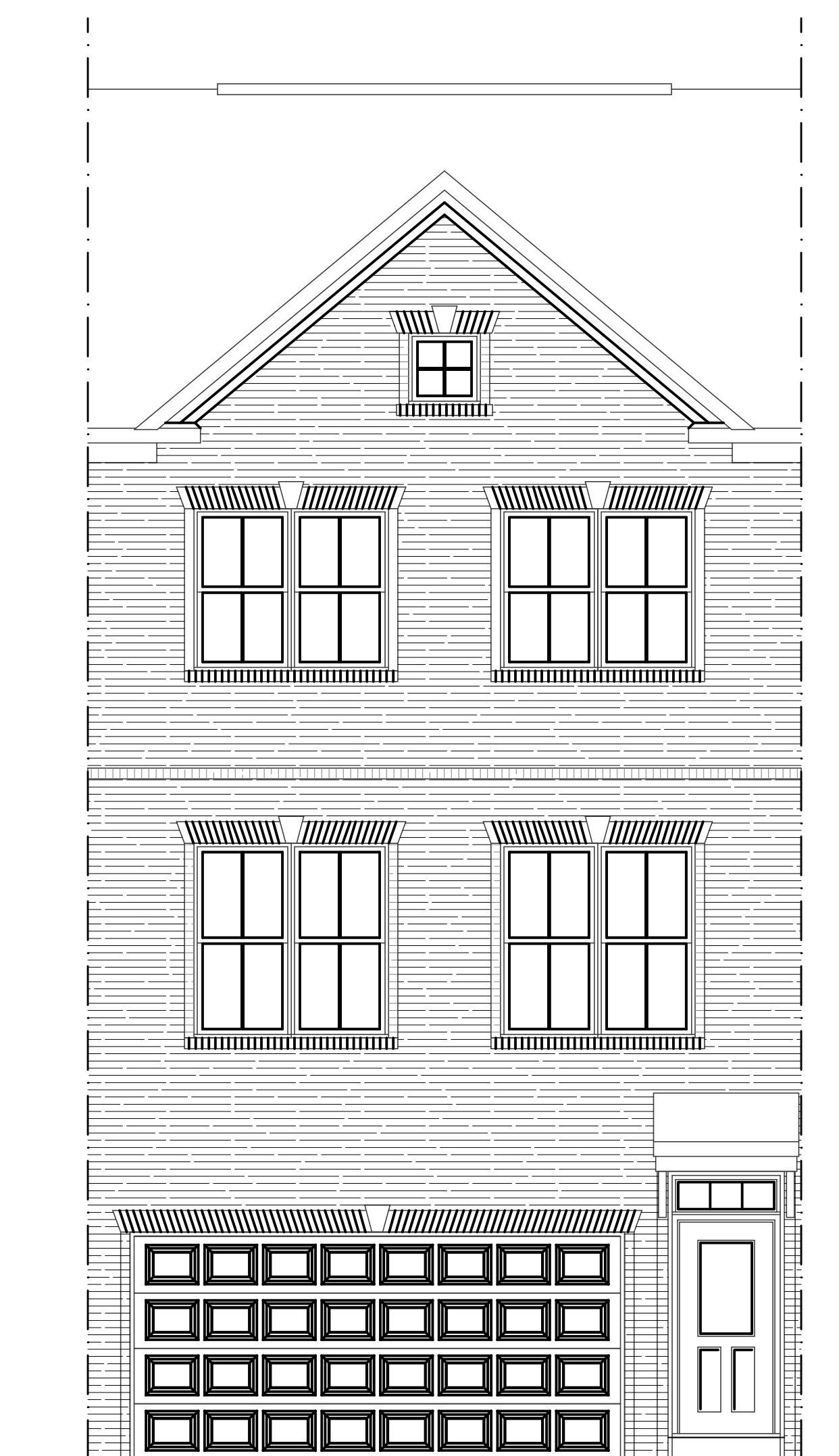
ELEVATION #4 UNIT 2450 FULL BRICK
